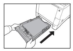
6 Insert the paper cassette into the slot in the machine. Push it straight in as far as it will go.
